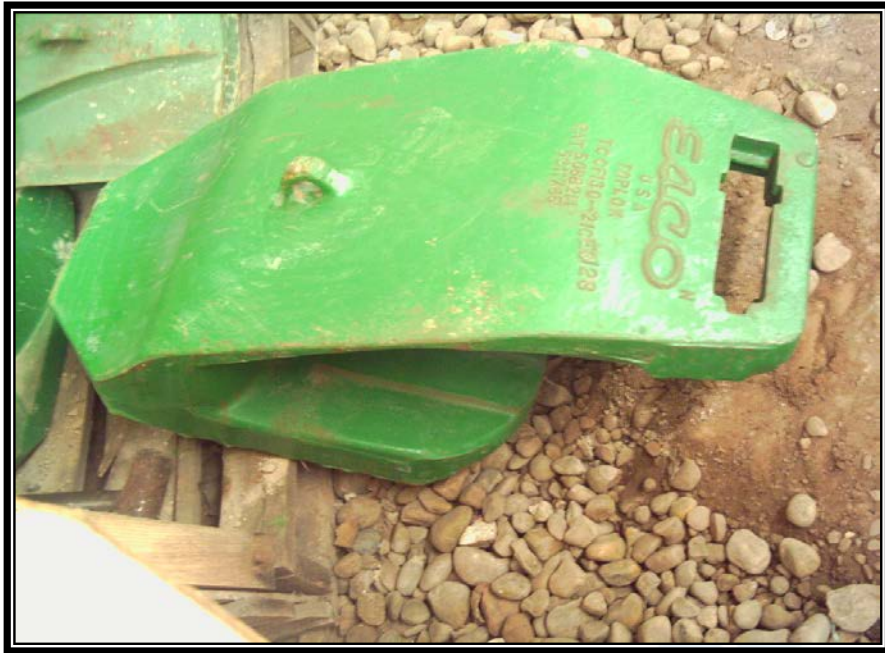
ESCO lip protector before being hardfaced with MIG Carbide
