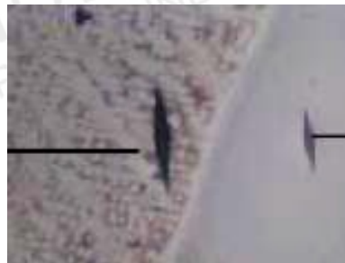
Hardness impression is a PS-98 Matrix 58Rc
