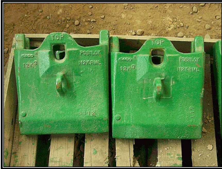
ESCO Shovel Tips before being coated Yanacocha Mines
