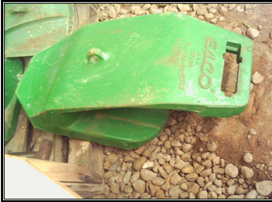
ESCO lip protector before being hardfaced with MIG Carbide Yanacocha Mines
